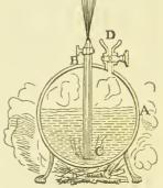
and both of the stopcocks shut, is placed over a fire, and vapour is generated in the upper part of it. This elastic vapour, pressing on the surface of the water, will, upon the opening of the stopcock H, raise it in the ascending pipe, and force it out at its orifice in the form of a jet d'cau.
